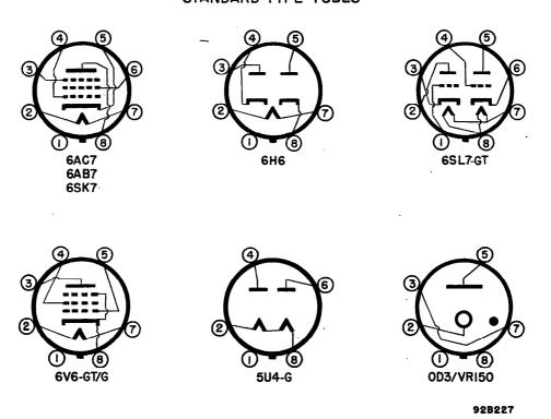
Figure 7-6. Radio Receiver Model S-37, tube socket connections.
